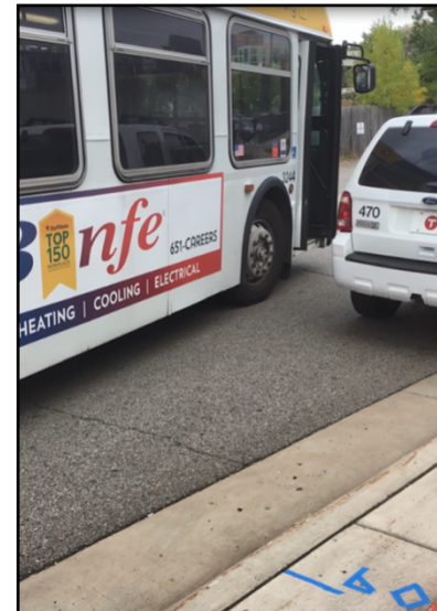
Figure 51 Screenshot showing a 60' bus testing a 10' merge zone (too short) for a far side stop and failing
