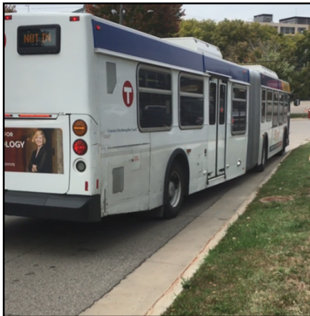
Figure 50 Screenshot showing a 60' bus testing a 20' merge zone (too short) for a near side stop and failing
