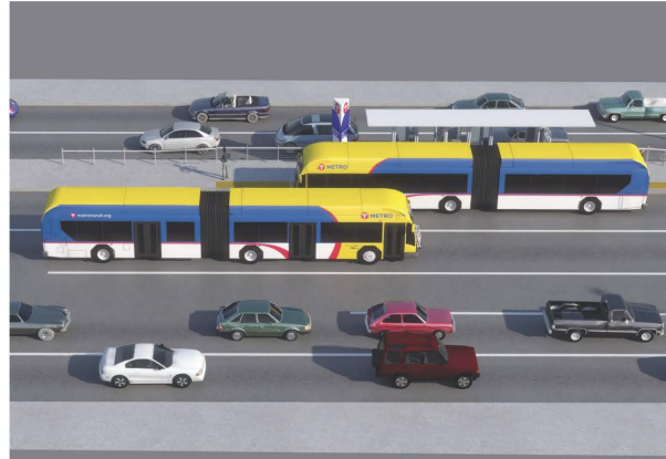
▲ BRT in bus-only lanes
