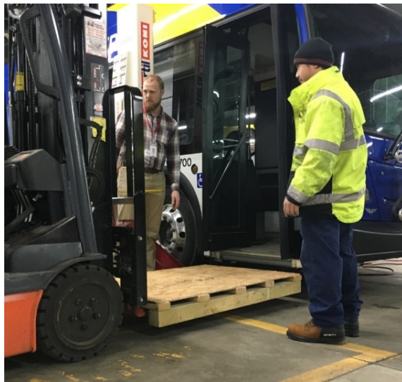
Simulated platform using forklift. Ramp deployment not successful at a 12-inch and 11-inch platform height.
