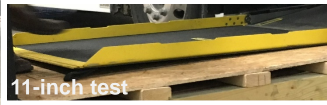
Simulated platform using forklift. Ramp deployment not successful at a 12-inch and 11-inch platform height.
