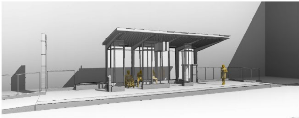
Figure 2. Plan sheet 8 and plan sheet 19 showing the front elevation of shelter Type 1. Type 1 shelters measure approximately 35' long and 11' wide.
