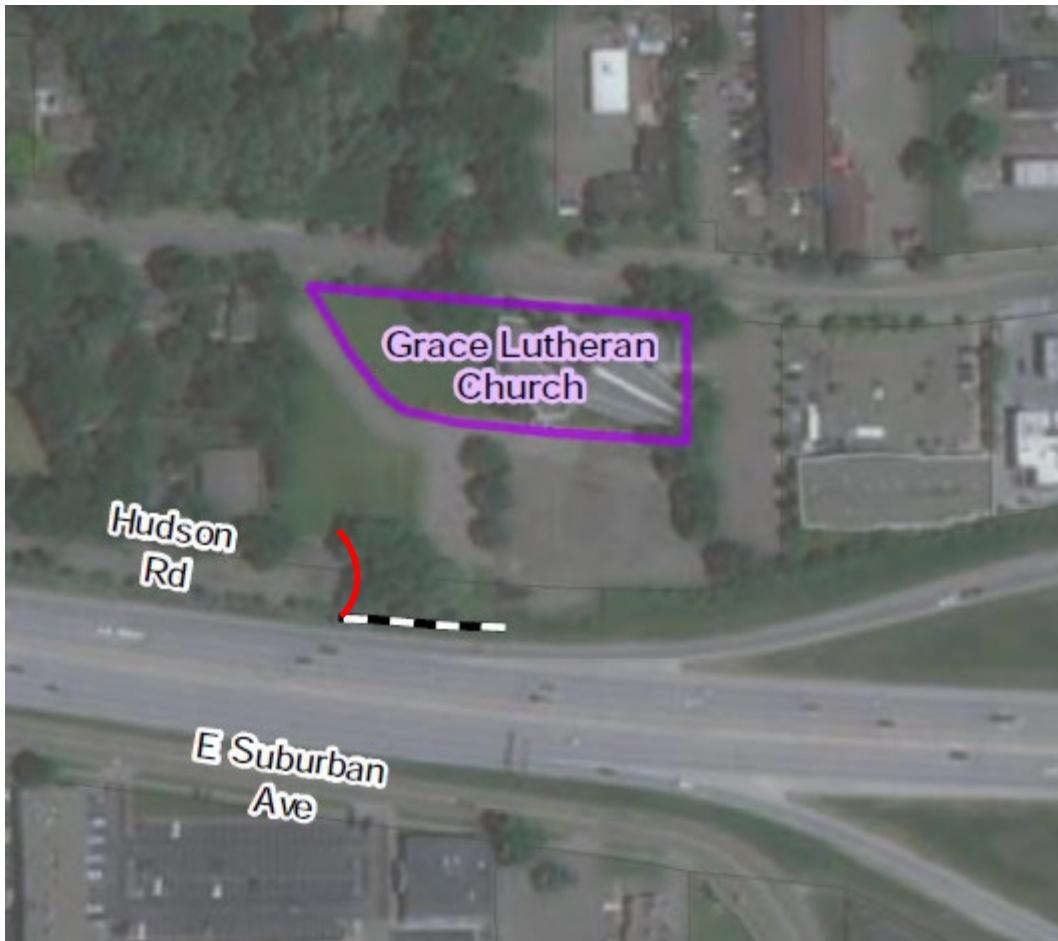
Figure 9. Proposed noise wall changes between 30% (red line) and 60% (black and white line) design. The purple polygon represents the historic property boundary.
