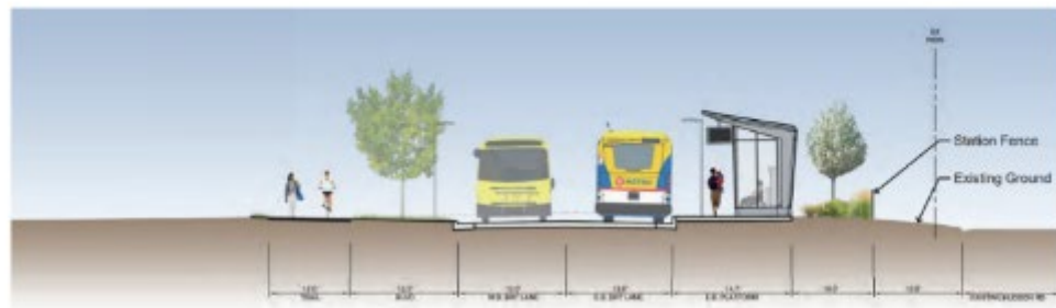
Section A-A: EB Platform (Looking East)
