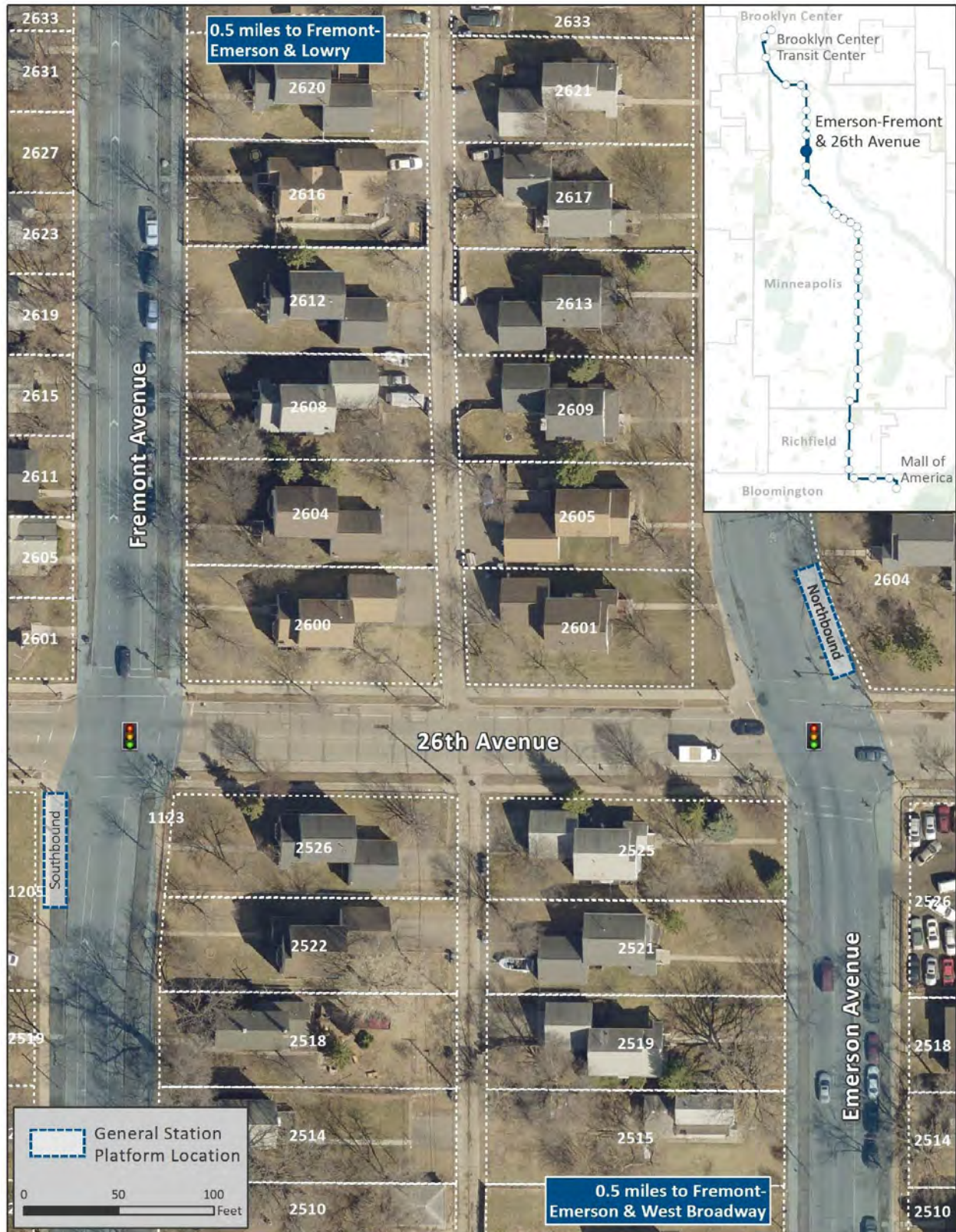
Figure 27: Recommended station location - Emerson-Fremont & 26th Avenue
