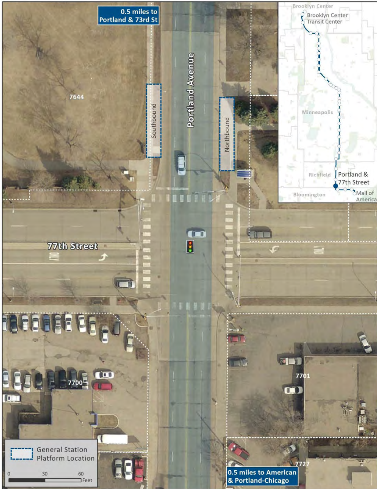
Figure 62: Recommended station location - Portland & 77th Street
